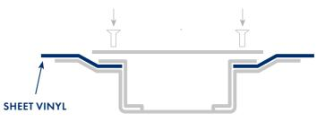
Only drains that have been specifically designed for use with sheet vinyl flooring should be considered in wet areas. These drains have clamping rings which prevent the ingress of water to provide a watertight finish.
