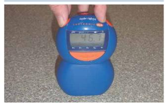
In order to cope with different contaminant spillages of various process materials, the surface roughness of the flooring must be sufficient in order to penetrate the squeeze films created when there is a presence of wet contaminants between shoe sole and the floor that prevents solid-to-solid contact. The surface roughness the floor requires is governed by the viscosity level of liquid contaminants in the application area.
